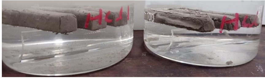
Figure 6 Specimens: HY 0.5 (left) and HY+15G 0.5 (right) after 3 weeks of exposure to 1% HCl (pH of 0.59)
